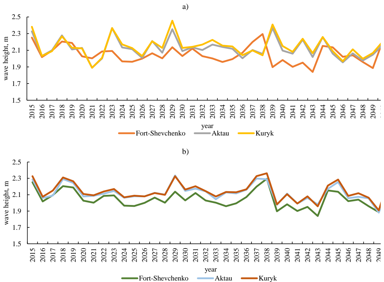
Figure 3. Projection of maximum wave height to 2050 under scenarios a) SSP1-2.6 and b) SSP5-8.5
